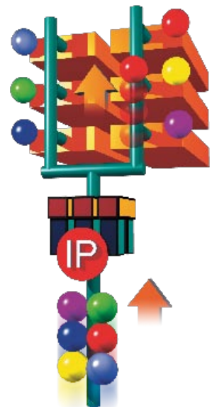
Figure 9: Traffic coming in from multiple IP addresses (represented by the colored balls) is distributed by the firewall amongst a pool of servers within the system. Unavailable systems will no longer receive traffic.
